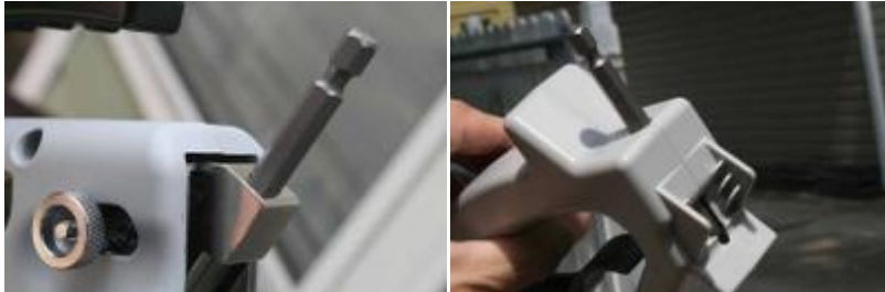
Notice how robust the marksman Pro is (left) compared to the all-plastic Marksman (right)
